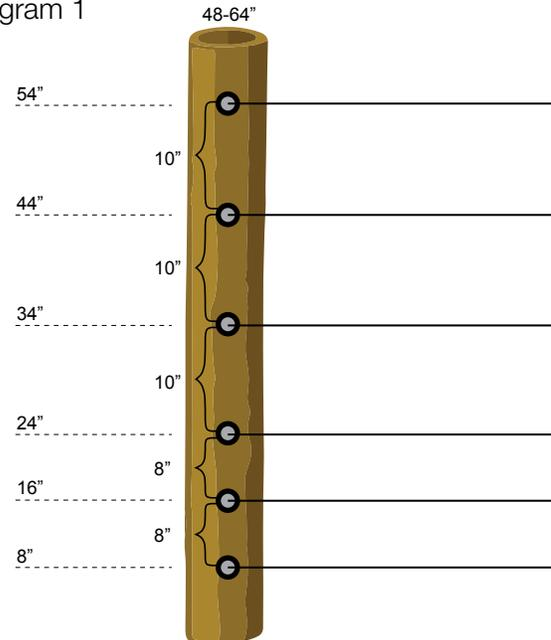
Wire spacing and height outlined here is critical in preventing low spots in the fence or large gaps between electric wires.
